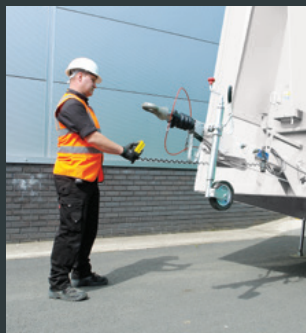
Unhitch from towing vehicle and operate hydraulics using the push button controls
